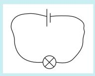
Provided that the electrical circuit is drawn correctly, non-rectilinear circuit diagrams are acceptable.
